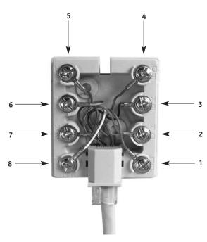
**Using the breakout box** A breakout box with a 3' CAT 5 patch cord (supplied) can be used to interface to the Phoenix system. Pinouts are shown in the tables and figures above.
